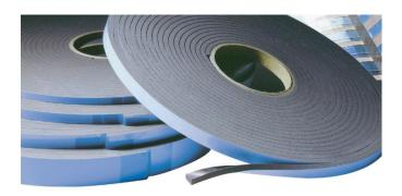
Single Sided high tack acrylic adhesive coated PVC structural spacer glazing tape. This tape is designed for use in structural spacer systems and has an open cell structure to allow the curing of structural silicones on all sides. Fast recovery from compression.
