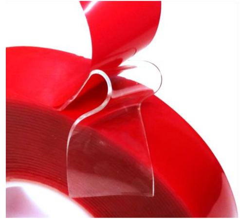
**QT562** exhibits extremely high adhesion and load bearing characteristics and is used in many industries for creating dynamic structural bonds. Bonds well to steel, aluminium, plastics, composites, ABS, PVC, HIPs, ceramics and glass. A permanent adhesive, designed to withstand temperatures ranging from -40 °C to +200°C. Good on textured and powder coated surfaces, also good on low energy substrates.
